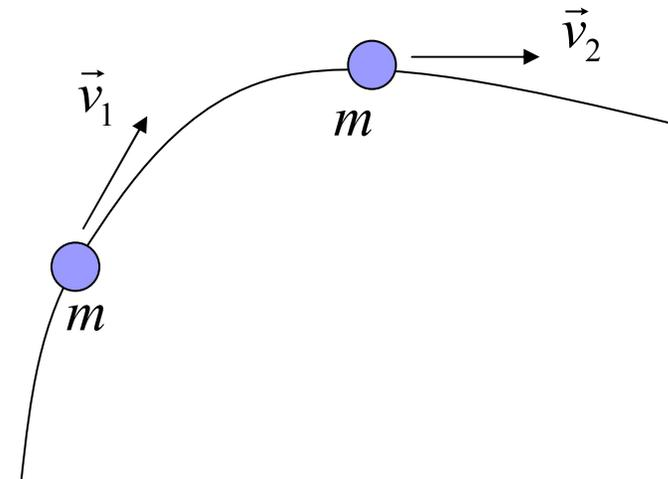
$$\vec{F} = m\vec{a} = m \frac{d\vec{v}}{dt} \frac{d\vec{r}}{d\vec{r}} = m\vec{v} \frac{d\vec{v}}{d\vec{r}}$$
